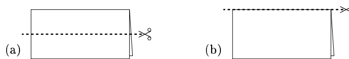
Fig. 5. Cut (a) can be made by a scissor cut, whereas Cut (b) cannot.
