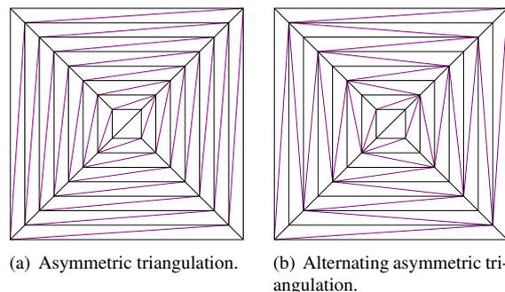
Figure 3: Two foldable triangulations of the hyperbolic paraboloid crease pattern (less one diagonal in the center).
