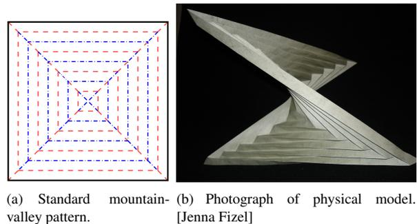
Figure 1: Pleated hyperbolic paraboloid.
