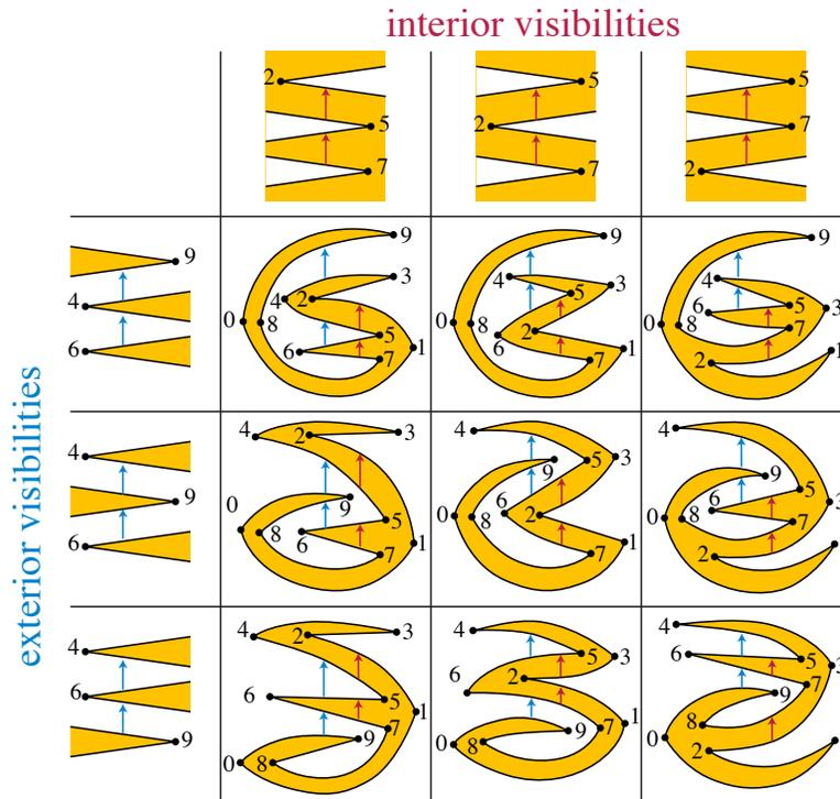
**Fig. 3.** A planar graph with two faces, each of which can be flat-folded to give three different patterns of vertical visibility (or “touching”) within it. These patterns can be combined independently, giving nine flat-foldings of the whole graph.
